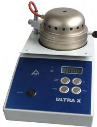
**This unique rapid incinerator was developed as a budget-priced alternative to kilns. It allows you to incinerate and ash single samples quickly and efficiently.**
